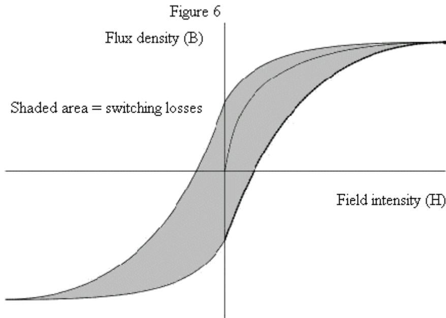
In order to return to the initial switched state, the remnance magnetism must now be overcome, hence input once in operation, will be greater than that required for the very first pulse. The area within the hysteresis curve gives a rough estimate for the amount of wasted energy, and along with other conventional sources of losses resultant in flux transfer within a core, is what reduces the efficiency of flux cores from maximum values of 2, or 4, down to values such as 1.75 or 3.47, typically.
