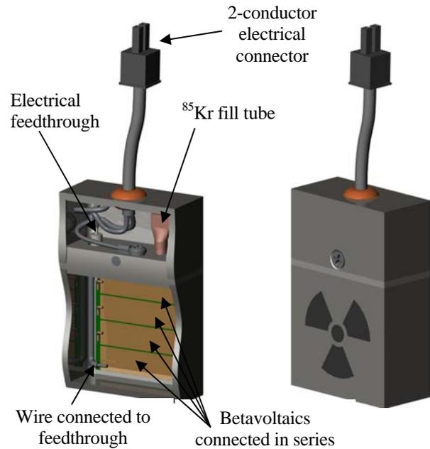
**Figure 3.** SolidWorks renderings of  $^{85}\text{Kr}$  QynCell and cutaway.
