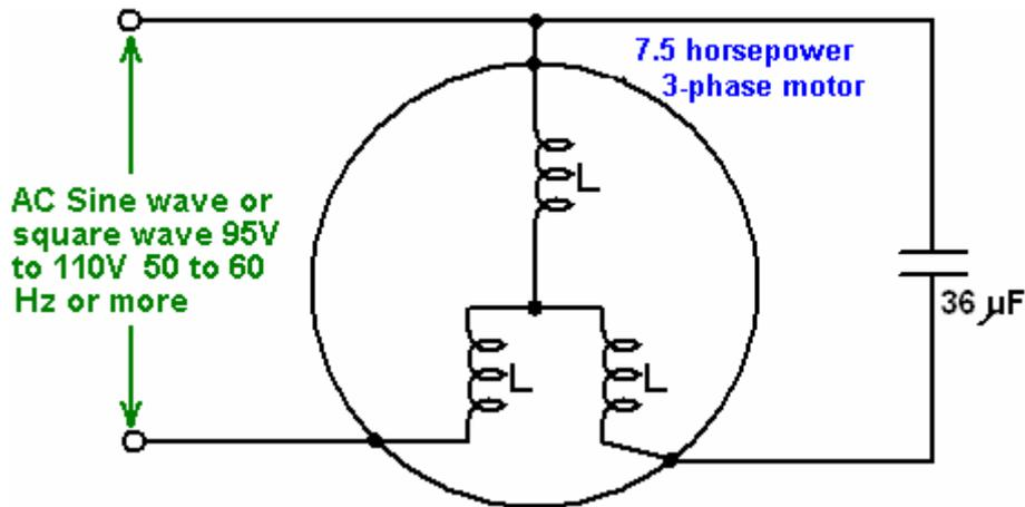
Because the running power draw is so low, it is possible to run this motor from a standard battery-powered inverter, but the current draw at start-up is some 17 amps, so the mains is used to get the motor started and then the motor is switched from the mains to the inverter. The inverter also allows easy measurement of the power input and so makes for easier calculation of the overall power efficiency of the system.
