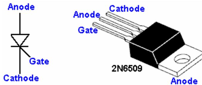
Please note that the 2N6509 package has the Anode connected inside the housing to the metal mounting tab.
