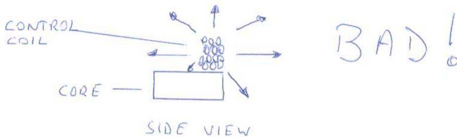
In picture 12 you see a side view of my setup. Only 30% of the core is active and the rest, as its not covered with the wires of the control coil, is not active. A very bad solution.
