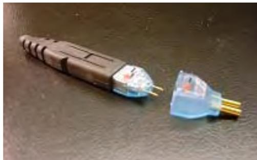
**Figure 14.** P7350 Differential Active Probe Plus Square Pin Adapter
