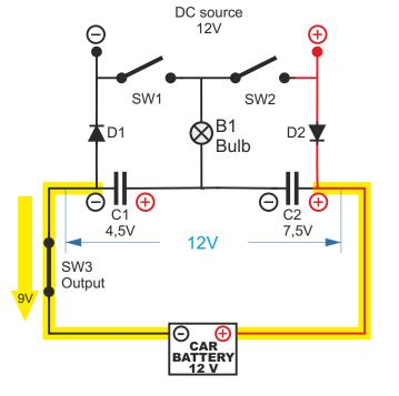
SW2 is closed, C1, C2 are emptying surplus 9V to battery. The energy from input is SAME as energy on output.
