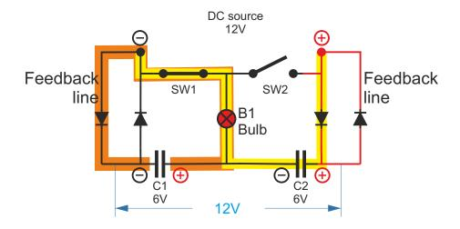
All the diodes in this configuration are not needed, feedback line is the same line used for filling capacitors.
