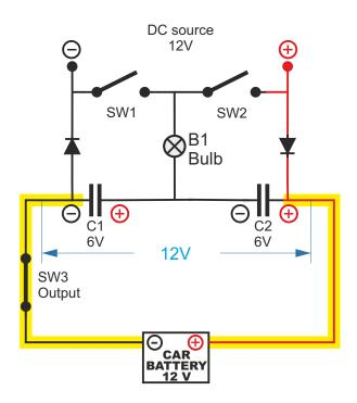
Fill both capacitors with 12V and then empty them in serial to battery. SW3 is closed, 1/2 of input Energy is dumped to battery.
