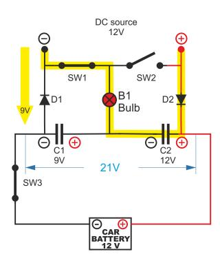
SW1 is closed, C2 is filled to 12V with additional 9V from input. Diode D1 **prevents** C1 to empty itself trough SW1.
