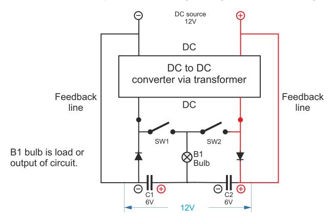
Solution for problem is to isolate feedback from rest of circuit. Diodes are needed to prevent C1 discharge through SW1 nad C2 through SW2. In this case with AC input switches are not needed.
