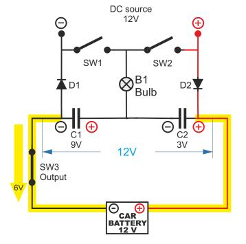
SW2 is open, C1, C2 are emptying surplus **6V** to battery. The energy from input is **SAME** as energy on output.
