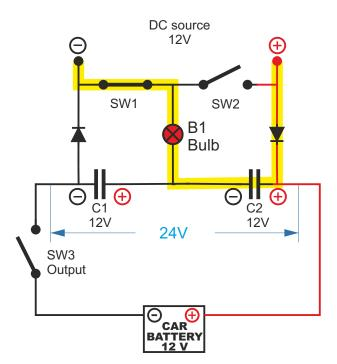
SW2 is closed, C1 is filled with 12V.
