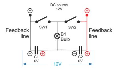
Solution for problem is to isolate feedback from rest of circuit. Diodes are needed to prevent C1 discharge through SW1 nad C2 through SW2.
