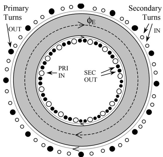
**Fig 4 – Toroidal transformer On No Load**
